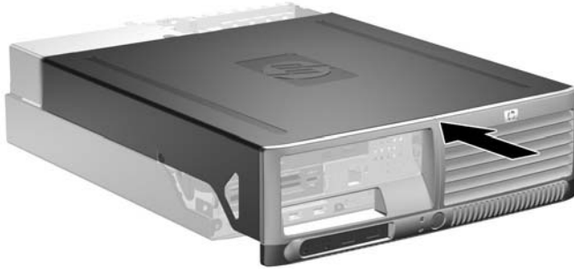
Figure 2-4 Replacing the Computer Cover
